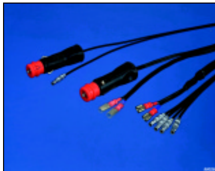
Fig. 9 (Left) Cables for powering NEXUS in a vehicle. From top to bottom: AO 0546 Supply cable with cigarette lighter to LEMO connector (3 m), AO 0547 Supply cable with cigarette lighter to spade terminals (3 m), AO 0548 Branched supply cable, spade terminals to 4 LEMO connectors (1.5 m); (Right) 19" portable rack (KQ 0158) that can hold 9 × NEXUS units (shown) or 8 × NEXUS units and a 32-channel Power Supply WB 1436 (not shown)
