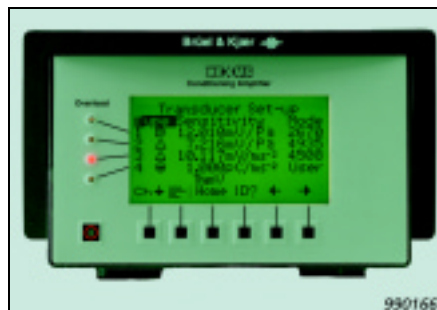
Fig. 10 Transducer set-up. Note that the sensitivity and mode fields have been automatically read from the IEEE P1451.4 compatible transducers
